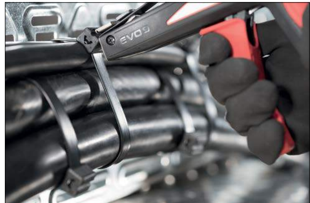
EL-TY series can be cut to suit any bundle with EVO9
